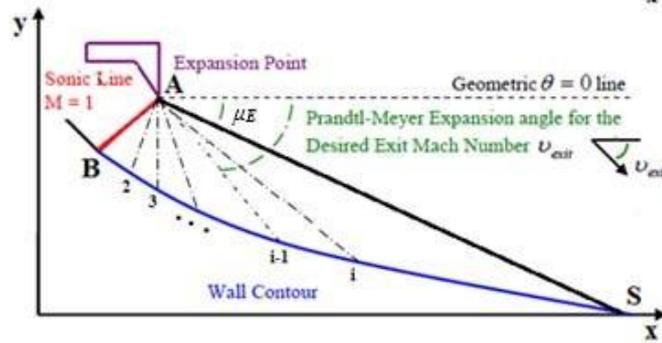
Figure 2. Generic geometry of a 2D plug Nozzle
