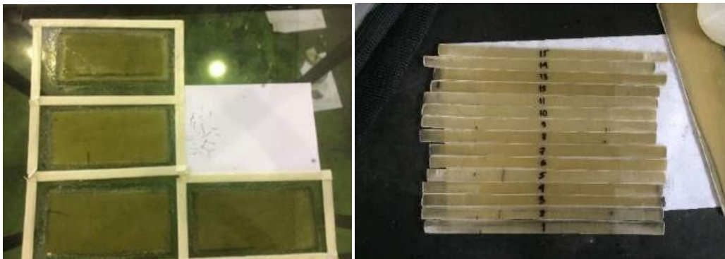
Figure 3. Hand Lay Up Specimens and Specimen Cuts
