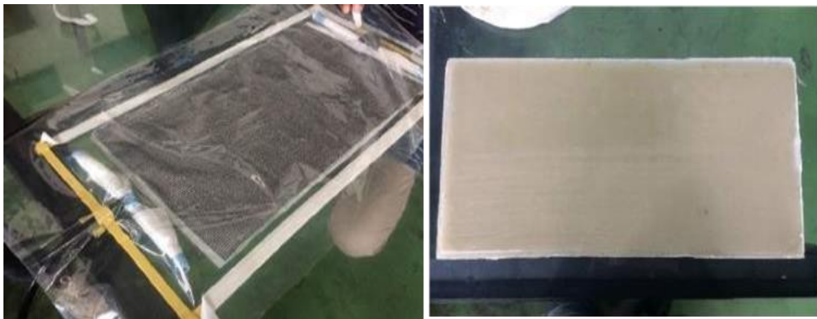
Figure 1. Vacuum Infusion Process and Vacuum Specimen Results
