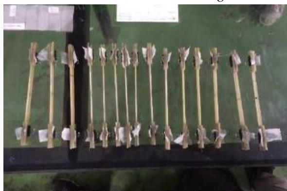
Figure 4. Specimens connected by Tab
