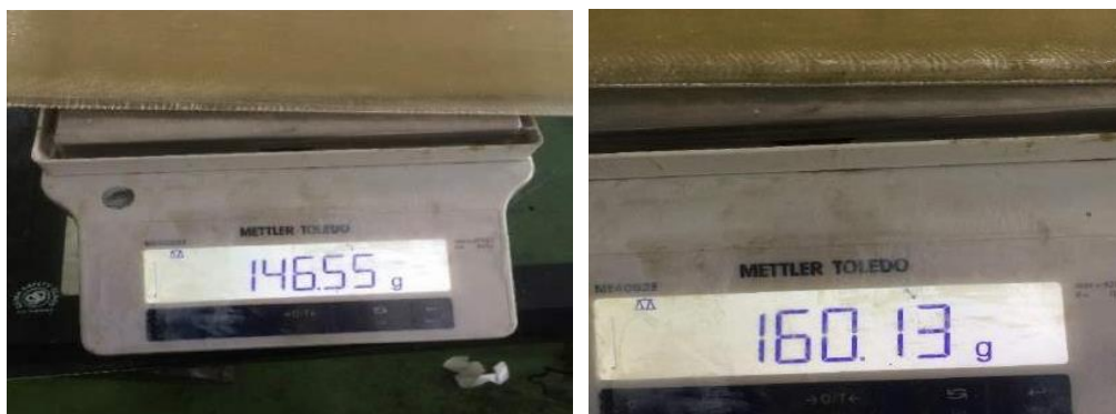
Figure 5. Mass comparison of composite specimens with vacuum infusion method and composite specimens with hand lay-up method
