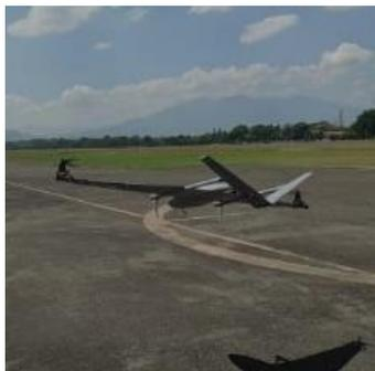
**Figure 15.** Aircraft gaining speed and transitioning to FW mode
