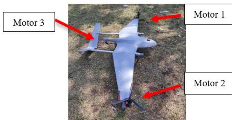
Figure 1. Aircraft Final Configuration
